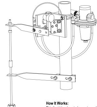
This liquid level control operates entirely by mechanical and pneumatic means. A float-operated air pilot valve controls the opening and closing of an air valve. It admits or exhausts air through a special regulator to turn an airoperated pump on or off.
